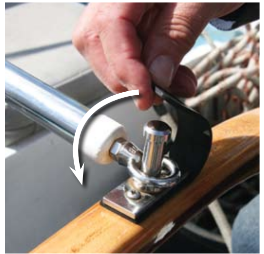
Above from left: A close up of the unit: Note the wooden back rest. The wide loop on the tiller arm drops easily over the tiller peg, and is secured from jumping off by a rubber collar.
