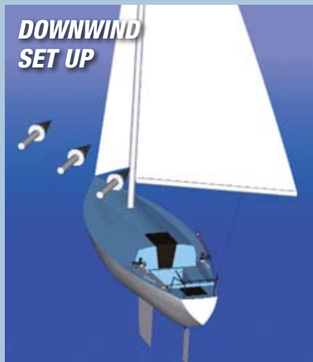
Sailing downwind. Spring and jib sheet are reversed, which takes some minutes to arrange.
